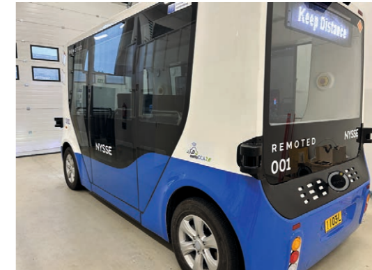
Image 23: The OHMIO LIFT vehicle with upgraded LiDAR and camera systems is being prepared for the operations at Remoted depot in Tampere. ©REMOTED / Tatu Nieminen
