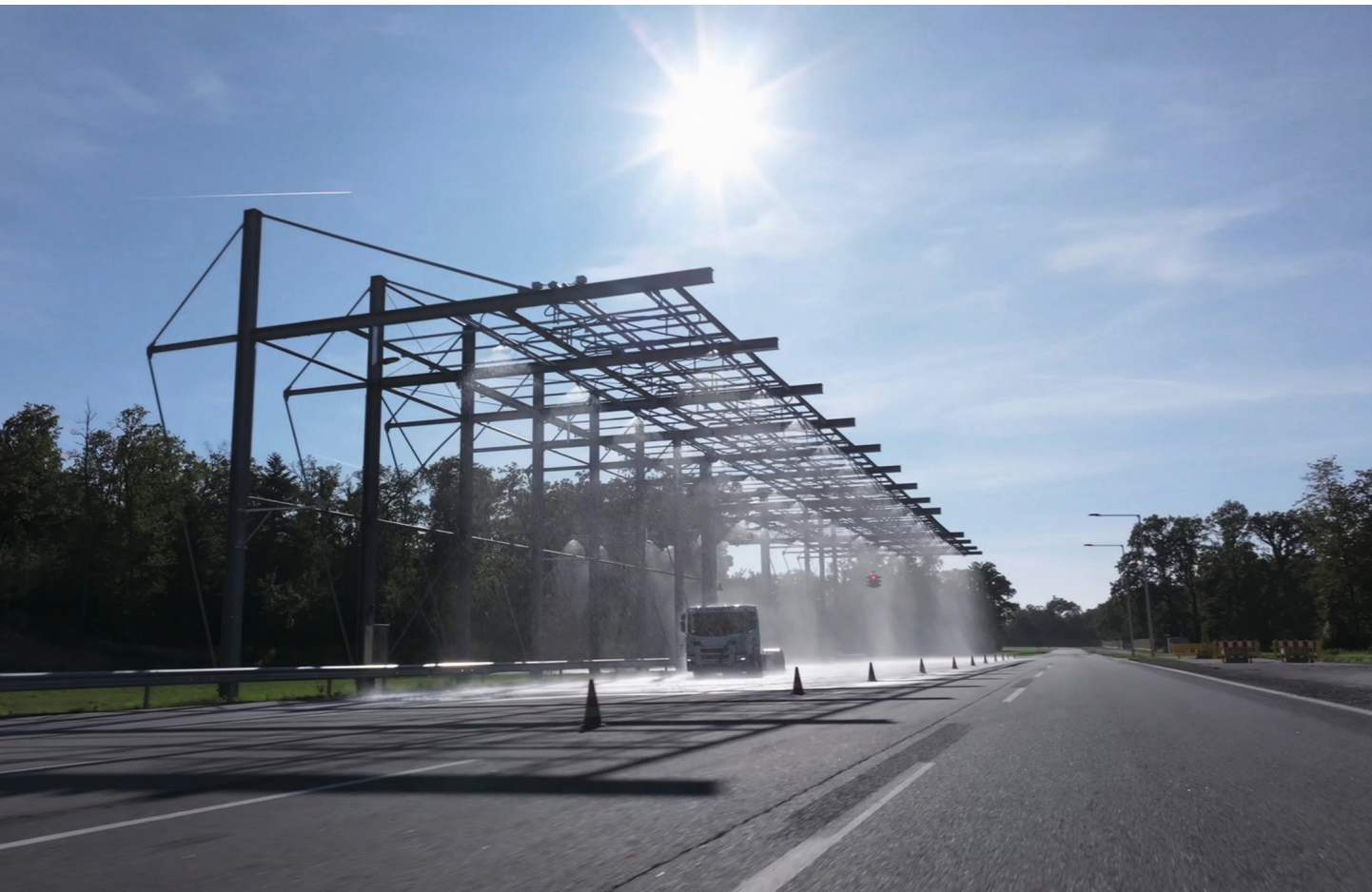
Image 4: Testing with the outdoor irrigation system in the Digitrans testcenter for automated driving in St. Valentin © Digitrans GmbH
