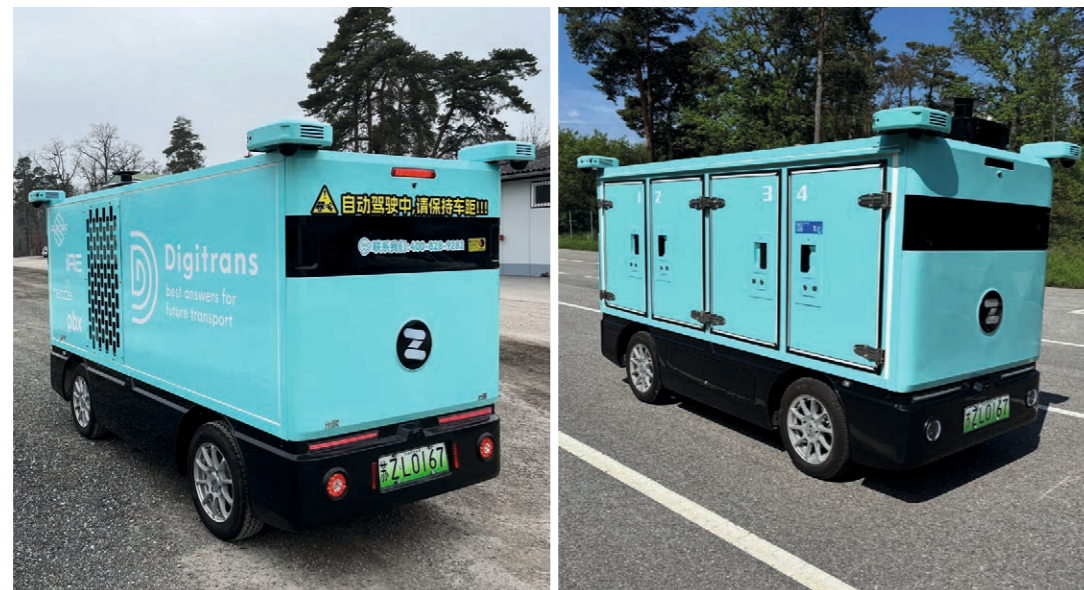
Image 5: Automated vehicle from China, which was extensively tested as part of the AURORA project, with view of the loading compartments ©DigiTrans GmbH
