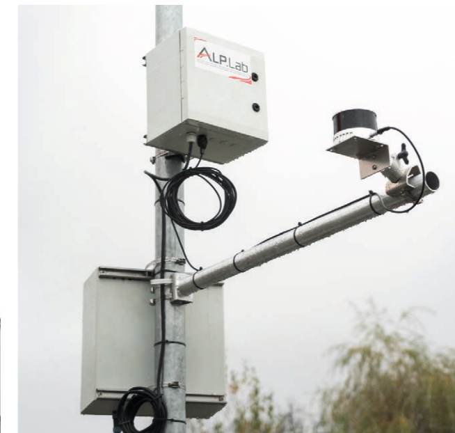
Image 9: The final sensor setup consisting of a lidar sensor, processing unit and battery © AustriaTech/Schallauer
